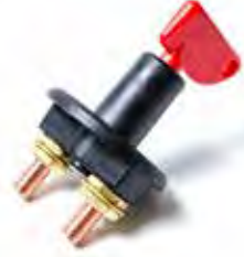
UN77310** BATTERY SWITCH Polyester housing is rust and corrosion proof. Removable plastic key for security. Two position switch "Off-On". Two 10MM X 1.5MM stud terminals. For panels up to 1.25 thick. Four mounting holes in a rectangle 1.3" and .8" on centers. 350 amp continuous rating. 500 amp intermittent rating.
