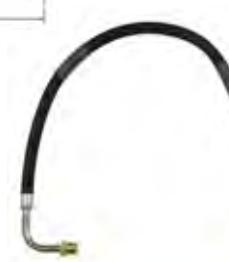
18-8115 FUEL LINE HOSE UNIVERSAL For fuel pump to carburetor connection. Replaces copper or steel tubing 3/8" X 25" PTFE composite hose with 5/8"-18 male inverted flare straight one end, 5/8"-18 90° one end. SAE J1527 type A1
