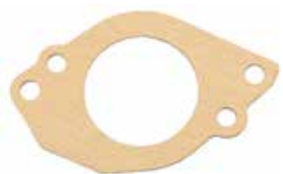
18-2472 CARB MOUNTING GASKET Replaces: 16221-ZW1-000 Fits: BF75(1997-06), BF90(1997-06)
