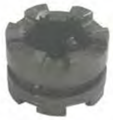
18-2383 SLIDING CLUTCH Replaces: 914716, 915272 For: 3.0L (GM), 4.3L (GM), 5.0L (Ford), 5.7L (Ford), 5.8L (Ford) (1990-91)
