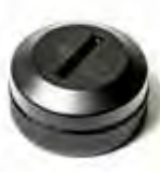
MP39190** WEATHER PROOF BOOT NUT Fits: All Sierra polyester ignition switches, 1996 & later. 13/16"-16 Thread. Rotating rubber seal. Seals out moisture and dust from lock cylinder
