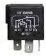
18-5705 POWER TRIM/FUEL PUMP RELAY Replaces: 582472, 584416, 586224 5 Terminal Single Pull - Double Throw - 12 Volt Open Contact: 40 Amps Resistive 30 Amps Conductive Closed Contact: 20 Amps Resistive 15 Amps Conductive
