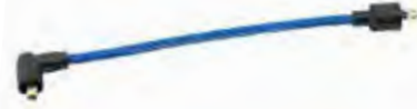
18-28102 COIL LEAD 12" long w/90 degree male Dist end and 180 degree male coil end
