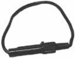
FS45350** FS45352 (Bulk 100pcs./carton) FUSE HOLDER • Black plastic twist lock case • 8" - 14 gauge wire loop • Includes 20 amp SFE fuse
