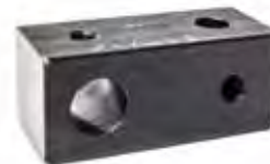
18-9866 DIAL INDICATOR HOLDING TOOL Replaces: Mercury Marine 91-89897 Description: Secures dial indicator to gear housing when checking backlash on MC-I, R-MR, Alpha One, TR, TRS drive units and outboards.
