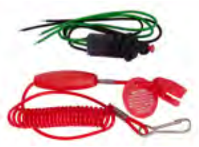
MP40950** EMERGENCY CUT-OFF SWITCH 4 terminals allow selection of normally open or normally closed circuit. Use MP40990 replacement lanyard.
