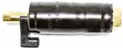
18-7326 ELECTRIC FUEL PUMP • 8 psi, 25 gpm Replaces: Mercruiser 805656A2, 805656A6, 805656A5, 805025A2, 861155A6, 861155A5 OMC/Volvo 3858261, 3850809, 3854620, 3857986
