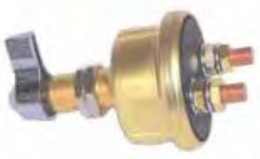
MP38910 LEVER OPERATED BATTERY DISCONNECT SWITCH Rated 175 A continuous, 800 A intermittent • 3/8" brass terminals • Chrome Plated Brass Lever • Includes faceplate
