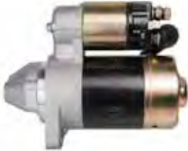
18-6936 STARTER Replaces: Yanmar 114361-77011, 114362-77010, 77011, 114399-77010 Fits: L40S, L60S
