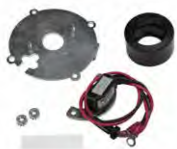
18-5294 ELECTRONIC CONVERSION KIT Fits: 6 Cyl. Delco distributors
