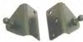
GS62880 Black zinc plated steel 90° angle bracket with 10mm ball stud. 2" x 1.2" base
