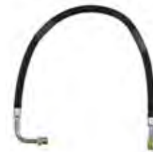
18-8115 FUEL LINE HOSE UNIVERSAL For fuel pump to carburetor connection. Replaces copper or steel tubing 3/8" X 25" PTFE composite hose with 5/8"-18 male inverted flare straight one end, 5/8"-18 90° one end. SAE J1527 type A1
