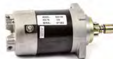
18-6417 OUTBOARD STARTER Replaces: 31100-92E00 Fits: 150, 200, 225 H.P. (1985-UP)
