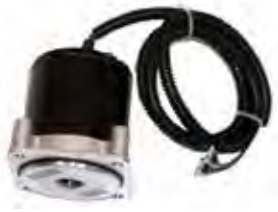
18-6783 TILT/TRIM MOTOR Replaces: 64E-43880-00-00, 64E-43880-01-00 2-wire ring terminal connection 4-bolt mount (O-Ring Included) For: 115-225HP (1997-2002)
